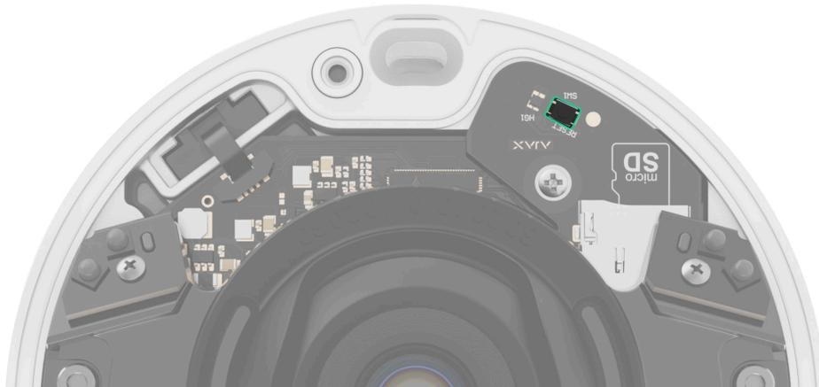
3. Power the camera while the reset button is pressed, and wait until the button's LED indicator lights up violet. This will take about 50 seconds.
