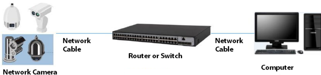
Figure 1-2 Connected through network router or switch
